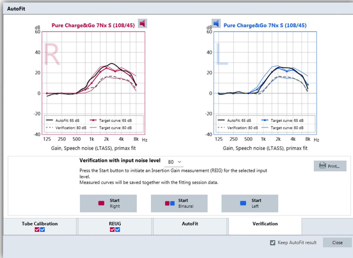
Figure 10: Insertion gain curves for 80 dB input signal, matching 80 dB targets.
