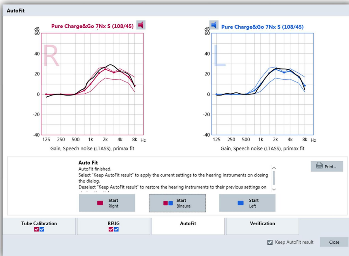
Figure 9: Insertion gain curves for 65 dB input signal after automatic fit-to-targets process
